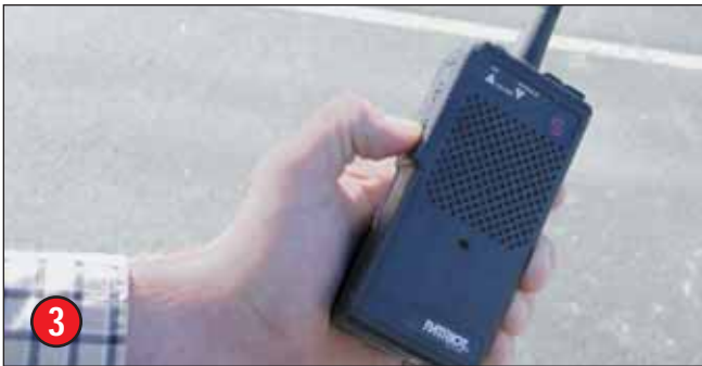
Call from gate is received via radio by facility personnel. Using a Ritron portable radio or desktop base station, authorized personnel can communicate remotely with individual at gate AND transmit a security code back to the OutPost wireless intercom/callbox to activate gate controller.
